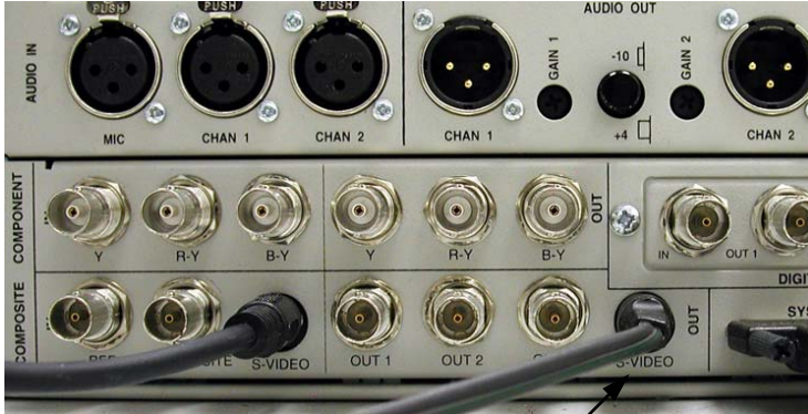
Connect S-Video cable to S-Video OUT Break Out Box
