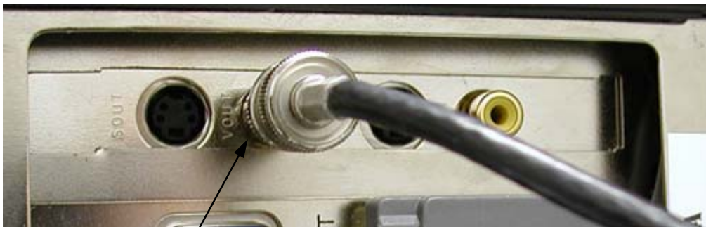
Connect composite cable to V OUT (left side)
