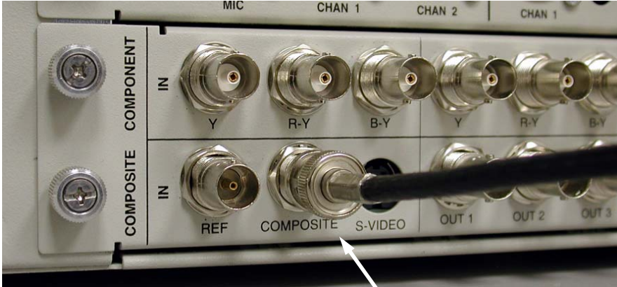
Connect a Composite cable from TBC OUT to Composite IN on Break Out Box
