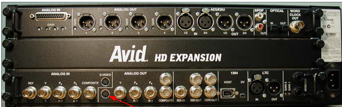
Connect S-Video cable to S-Video OUT on Break Out Box
