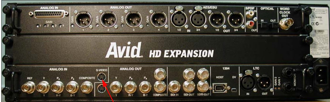
Connect S-Video cable from TBC OUT to S-Video IN on BOB
