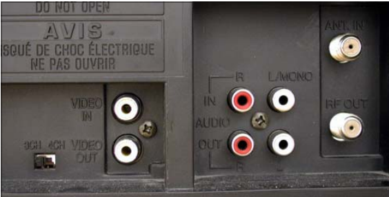
Use composite cables if your deck looks like the image above (see page 8)
