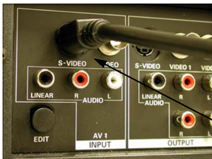
Connect S-Video cable from S-Video OUT on the BOB to S-Video IN on deck
