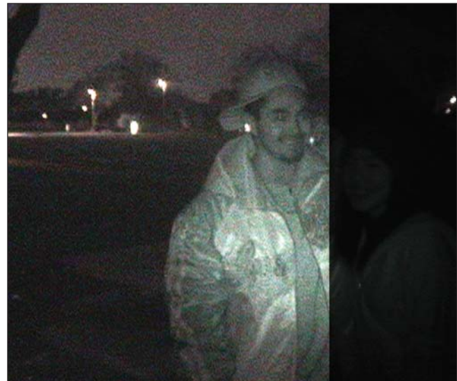
working on the video with the dTective System from Ocean Systems, Brown was able to obtain something useful (on the right). Notice that only the left side of this image has been enhanced through highlighting. The right side has been left unchanged to emphasize the difference.
