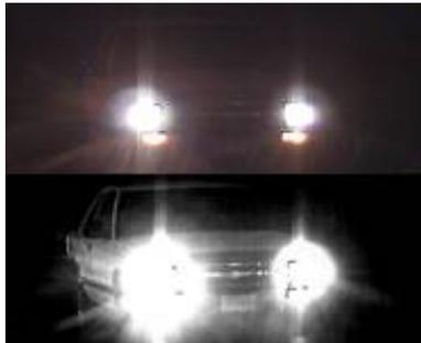
When dTective software processes grainy surveillance video (top), details such as license plates can be seen in the resulting images (bottom). (Ocean Systems)
